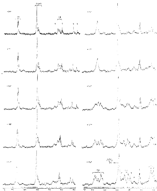
Figure 5. Nmr spectra (60 MHz) of cis -(1,2,6-trihapto:3,4,5-trihapto)cyclooctatetraene)hexacarbonyldiruthenium. An approximately 0.1 M solution in ~3:2 v/v mixture of \text{CD}_3\text{C}_6\text{D}_5\text{-CF}_2\text{Cl}_2 . The peak marked T is due to toluene- d_7 and peaks marked X are due to impurities. Numbers indicate assignments as represented in Figure 6.
